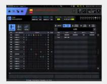
Includes a summary monitoring screen and gives the operator easy access to DN Solutions's own tool management system which provides comprehensive real time data on each tool, such as remaining tool life and status of tool groups.
